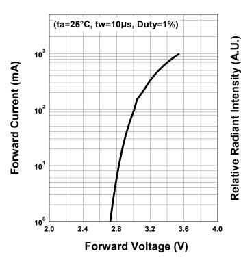
Relative Radiant Intensity - Forward Current
